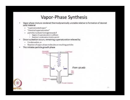
These are examples of nano-particles or nano materials that are obtained by taking two reagents and mixing them together at molecular scale to produce a nano dimensional material. Vapour phase synthesis on the other hand is one, where you essentially saturate the vapour phase with the nano material that you are trying to synthesize and then, you actually make it thermodynamically unstable and with leading to the formation of the desired material.
