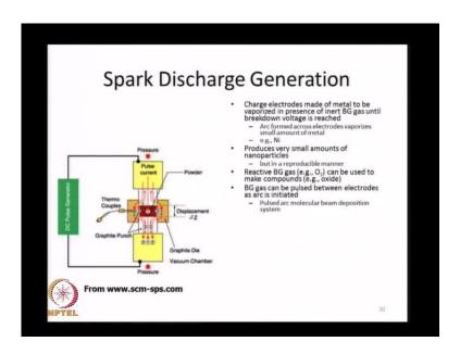
Spark discharge generation is another technique to take solid metal and vaporize it. So, here you essentially make electrodes of the particular metal to be vaporized and you charge them in the presence of an inert background gas, until you reach a breakdown voltage. Above that voltage an arc forms across these metal electrodes and vaporizes a small amount of the material which can then be used to make nano-particles of that material example is nickel.
