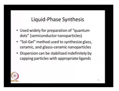
Now, liquid phase synthesis is a slightly different technique. The most common example of it is the Sol-Gel method; it is used for preparation of quantum dots which are semiconductor nano-particles. The method can also be used to synthesis glass, ceramic as well as glass ceramic nano-particles.
