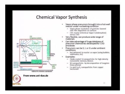
Chemical vapour synthesis is probably the most widely used method to make nanoparticles in the bottom-up approach. Here, you take vapour phase precursors and you bring them into a hot wall reactor under nucleating conditions. So, essentially this is a reactor in which there is a target surface, but even though walls of the chamber are heated to high temperatures, because of this the entire reactor is in a condition where it promotes nucleation.
