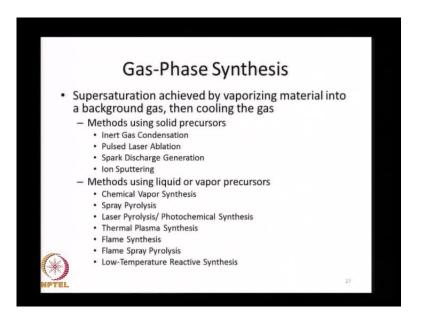
Now, gas phase synthesis is actually very similar to what we are termed earlier as vapor phase synthesis. The difference here is, you have a background gas into which your vaporizing material and the super saturation here is achieved by vaporizing a material into a background gas and then providing appropriate cooling of the gas to achieve the super saturation.
