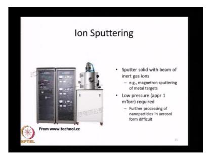
Ion sputtering is another commonly used technology where in this case, you are essentially impacting the solid surface with high energy ions. So, this process is called sputtering.
