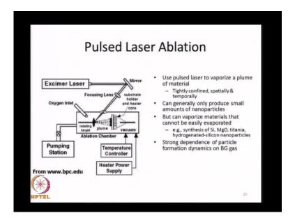
Pulsed laser ablation is another way to vaporize material. So, for metals that cannot be vaporizing simply by heating, you hit the metal surface with high energy laser and it vaporizes essentially a plume of material. Some of the advantage of this technique is, it can be very localized, you can hit certain geometries on the surface and vaporize the material only in that area. So, it is tightly confined both spatially and temporarily.
