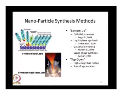
So, what are the two basic types of synthesis methods? Bottom-up and top-down, the difference between the two is that, in the bottom-up approach essentially you take atoms or molecules and you tie them together to make nano materials.
