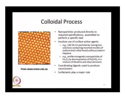
Let's talk about some of the bottom-up approaches, first what is a colloidal process? In this process, essentially you build up the nano material and atom at a time. So, you take the specifications that have been laid down for properties of the nano material and you take nano-particles and assemble them in a certain way to be able to meet these specifications, in order to be able to perform a specific task.
