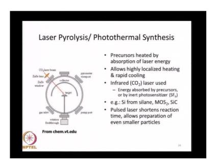
A related technique is laser pyrolysis or photothermal synthesis. Here the precursors are heated by absorption of laser energy and this technique allows highly localized heating and rapid cooling. So, quenching becomes easy when you are using this technique. You do not have to allow growth to occur beyond a point where you want to stop it. Infrared laser, C O 2 laser can be used which reduces the expense of the operation.
