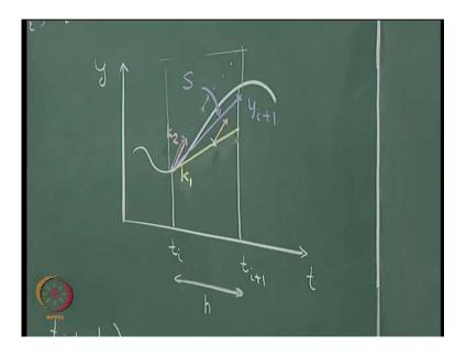
So, the third point will lie in that particular rectangle and find the slope at that particular point k 3. And another point - fourth point - will also lie in that another rectangle so constructed and that slope will be k 4, and the final S that we are going to use in order to compute the term y i plus 1 is going to be a weighted sum of k 1, k 2, k 3 and k 4. The most typical r k - 4 method that is often used has w 1 equal to 1 by 6; w 2 and w 3 equal to 1 third; and w 4 equal to 1 by 6 again.
