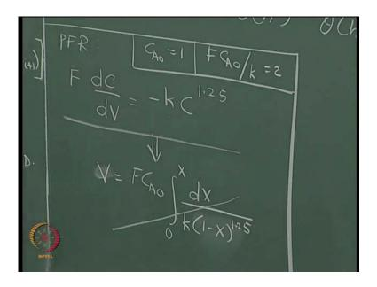
So, now, what I will do is, I will go on to Microsoft excel and solve the specific problem of the p f r. The p f r problem, the design equation that we had solved; we had obtained the design equation based on the overall equation d c by f multiplied by d c by d v, where f is the flow rate - volumetric flow rate - that is going to be minus k c to the power 1.2 5.
