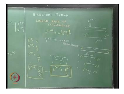
So, these are essentially true two important expressions to keep in mind; this particular way of convergence is what is known as linear convergence; so, the bisection method has a linear rate of convergence; what we mean by linear rate of convergence? Or in general, what we mean by rate of convergence, is how our E i plus 1 is related to E i; so, E i plus
