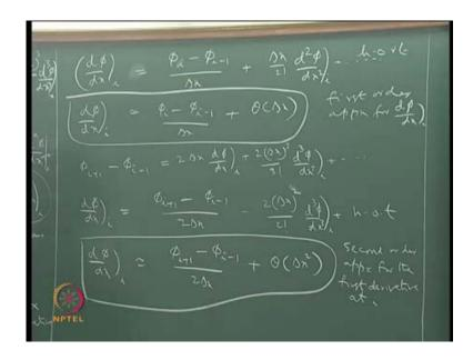
Now, if you were to write it as a first order or a second order like this, we can see that we can therefore write at d phi by dx at i roughly as phi i plus 1 minus phi i minus 1 by 2 delta x plus terms of the order of delta x square, because the leading term in the truncated series here has a square term associated with delta x. So, this is therefore, we call this as a second order approximation for the first derivative at i.
