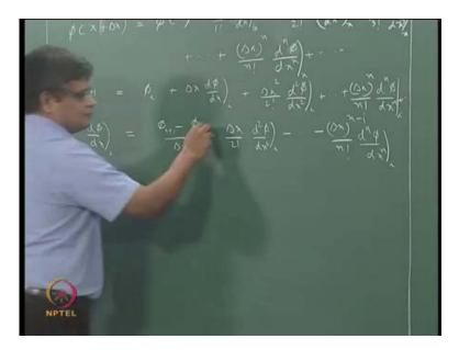
So, from this, we can write an approximate formula for this. We can write therefore, from this, d phi by d x at i is equal to phi i plus 1 minus phi i by delta x. So, I take all these things on to the left hand side and then I divide by delta x here minus delta x by factorial 2. This square here will cancel with this, so, I have d square phi by dx square at i minus, minus delta x n minus 1 by factorial n d n phi by d x n like this.
