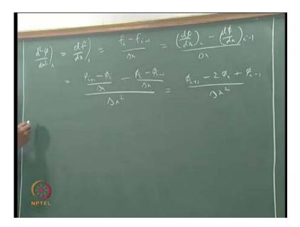
And we can use, we can use, we can, for example, do it in a different way d square phi by dx square at i is d f by dx at i. For example, we can write this as f; we have made use of backward differences here.
