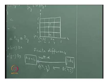
So, the objective is to go from phi x y to phi x i y j so that to, in order to find these values, we need to solve only an algebraic equation, a set of algebraic equations, not a partial differential equation.
