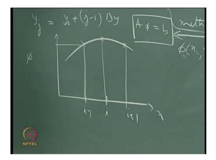
Let us say that this is the variation of phi with respect to x and we are looking at discrete points like i here i plus 1 and i minus 1. So, the value of phi, this is the value of phi i minus 1 and this is the value of phi i plus 1 and this is the value of phi at i and what we are interested is not specifically the value of phi, but d phi by dx.
