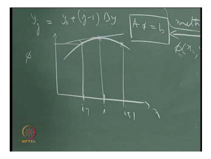
So, we are looking at the slope and the slope at this point is maybe something like. This, this, is a true slope by expressing in terms of i plus 1 minus i by delta x. We are evaluating a slope of a line which is passing through these points.
