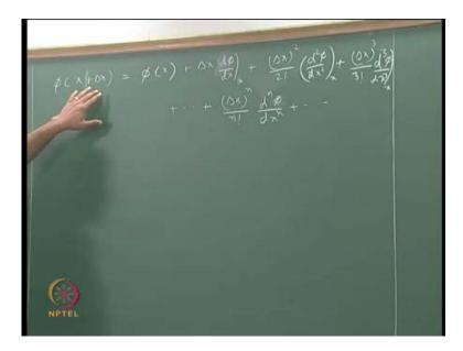
So, the idea is very simple. If you have phi of x, so, let us consider the case of onedimension and we are looking at a function phi of x, and so, phi of x plus delta x, that is, the value of the function at a point which is slightly displaced from x can be expressed in terms of the function at x in the following way using the Taylor series approximation.
