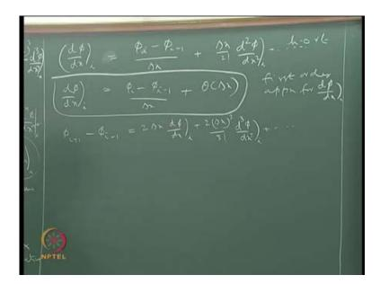
So, we can say that phi i plus 1 minus phi i minus 1. If we do this, then this and this cancels out and we have delta x d phi by dx at i minus delta x minus delta x this. So, when we subtract this minus becomes plus. So, we can have we will have 2 delta x d phi
