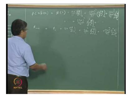
So, we can say that, so, if phi of x is phi of i, then x plus delta x, that is, one grid point away can be expressed as phi i plus 1 is equal to phi i plus delta x times factorial 1 and i plus delta x square by factorial two times d square phi by dx square at i plus delta x raised to the power n by factorial n d n phi by dx n evaluated at i and so on like this.
