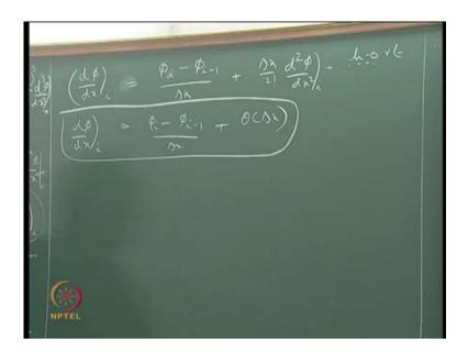
So, that is equal to phi i minus delta x d phi by dx at i plus delta x square by factorial two d square phi by dx square at i plus higher order terms, and using this expression, we can derive an approximate formula like this for the first derivative phi i minus phi i minus 1 by delta x plus delta x by factorial 2 d square psi by d x square at i plus so on plus higher order terms.
