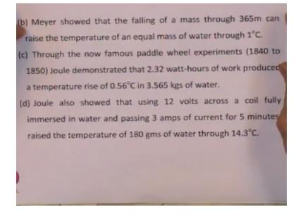
Second experiment which was to Meyer who showed that the falling of a mass through 365m can raise the temperature of an equal mass of water through 1°C. Now the third experiment consists of the same of paddle wheel experiments by joule between 1840 and 1850 who demonstrated that on an average 2.32 watt-hours of work produced at a temperature rise of 0.56°C in 3.565 kgs of water.
