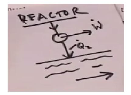
Let us say you have a river flowing, you have a nuclear reactor. So you are drawing heat from it, you are rejecting heat here, and you are doing work here. And this W is related to this amount of heat rejected here or W. is related to Q2 part.
