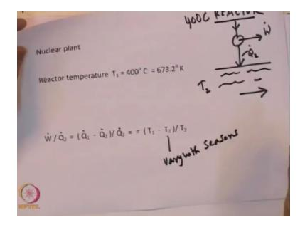
And you go back to Carno, Carno tells you that this reactor here in this case there is 4000C and this temperature varies with the season here this is T2, so if the reactor temperature is T1 it is equal to 673°k. Now W/Q2. Is if you like Q1.-Q2./Q1., but this is equal to T1-T2/T2, that is what Carno has told. Now T2 can vary with season, so you are asked to calculate in two seasons what is the amount of work that power you can produce. The dry season flow rate is given as 2m3 per sec.
