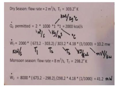
And the temperature you already being told 30° which is 303.20k. So you can use this formula you know W./Q. is simply Q1-Q2 IS W./Q2 which is T1-T2 /T2. So if Q2. permitted is now given to you it is given as 2x1000x1 this is simply m<sup>3</sup>/sec this is kg/m<sup>3</sup> for water, this is the specific heat which is kcal /kg°C in the thermal pollution allowed is 1°C. So if you multiply these out you get 2000kcal/s this is the permitted thermal pollution.
