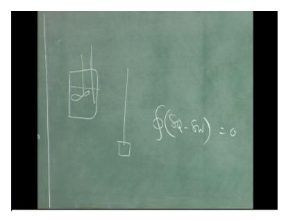
But in mechanical system, thermo mechanical systems he showed that the cyclic integral of delta Q- delta W = 0 although the cyclic integral over delta Q itself or delta W itself was never 0, so Q and w are functions of path but the difference is independent of path, therefore he said this quantity can be called a perfect differential and he wrote this is du.
