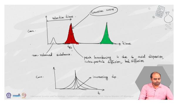
You would get a pulse input sorry pulse output in the chromatographic or the chromatogram that you analyze at the exit. But normally this is known as a perfect pulse, but normally that is not achieved. So, this whatever the output that is seen is generally broadened because of axial dispersion or diffusion. So, this peak broadening, is due to axial dispersion, intra particle diffusion, then you have this axial dispersion or bed
