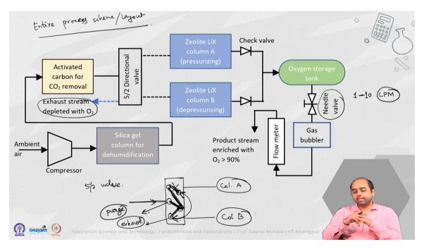
So that you know this the requirement of pressurization or the requirement of high pressure step during adsorption is reduced. So, normally the operating pressure for this you know system is around 2 bar gauge pressure. So, if you apply vacuum even you can operate it at 1.5 bar also of course, in gauge pressures I am talking about 2 to 2.5 is
