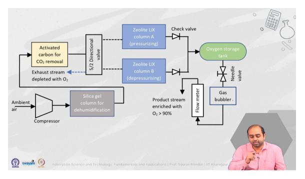
So, in that case column B is actuated through this line where this is I mean this is like the exhaust connection right. Now when column B and this is the exhaust connection and this
