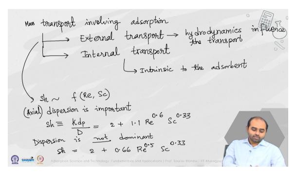
So, in the external transport, hydro dynamics influence the transport. So, typically the external transport case is defined by Sherwood relationships and this is a function of the Reynolds number and the Schmidt number of the system. So, typically for experiments
