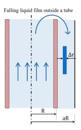
Whereas, when the liquid reaches the top of the tube, obviously it is going to spill over. So, it is going to spill and it is going to fall along the walls of the tube, along the outer walls of the
