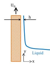
An upward moving belt, with a velocity equal to Uo, drags a viscous solution along with it creating a thin film of thickness h, as shown in the figure. Obtain an expression for the liquid velocity in the film, in terms of the relevant parameters.
