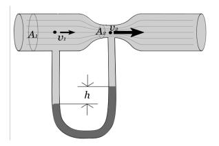
So, that means the pressure goes down, and pressure goes down up to the throat, and then pressure is supposed to recover beyond the throat. So, the pressure versus distance you have this type of a plot. So, this gives you a very unique opportunity to reduce pressure at the throat and then the question is how far it will go down. I mean if you have it depends on the ratio of A1 and A2 right what A1 by A2 you have.
