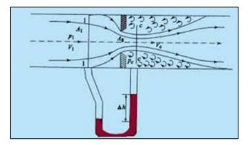
So, this is inexpensive easy to fabricate, but comes with the high or rather low value of C high pressure head loss at this point. So, this is called the orifice meter. So, high head loss low cost suspended matters may start to build up. There is a third kind of flow meter which is a variable area meter it is known as rotameter. So, what you have is a float and in the rotameter the area diverges like this and you have flow from the bottom.
