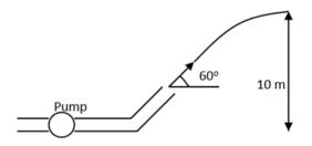
So, one we can assume that the jet starts from the level and it must reach the 10-meter height building. So, for do not consider this part the height of this part. So, we can assume that the water has to reach to a height of 10 meters. So, a fire personnel mistakenly picked a nozzle whose diameter is the same as that of the hose.
