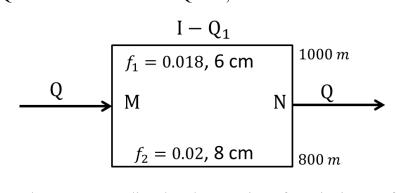
So, in this example one must realize that the equation of continuity can first be used. The equation of continuity essentially tells us that the sum of the flow rates in the 2 branches Q1 and Q2 must be equal to the overall flow rate which is 20 Liter per second. And if you divide Q1 and Q2 express Q1 and Q2 in terms of velocity and area. So, this is going to be A1 v1 plus A2 v2 is the total flow rate. So, this is nothing but the equation of continuity.
