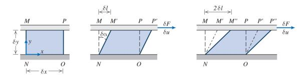
Here I have two plates: one is this one, and the other is this one. So, the lower plate is fixed, and the upper plate is moving. The gap between the two plates is given by  $\delta y$  and this is the x and y direction. So, I am focusing on this element, which is MNOP, which has a dimension  $\delta x$  in this direction, and  $\delta y$  is in this direction. So, now if the upper plate moves at constant velocity  $\delta u$ , under the influence of constant force  $\delta F_x$ .
