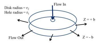
The pressure is  $p_1$  at  $r = r_1$  and  $p_2$  at  $r = r_2$
