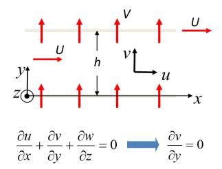
So, here because of fully developed condition del u del x is going to be equal to 0. Since the flow is fully developed u is not a function of x. So, this term would disappear there is no there is no flow there is no velocity in the z direction. So, w the z component of the velocity is 0 which leaves us with del v del y to be equal to 0 which essentially gives me v is a constant and or v could be 0. Now, we know that v is equal to capital V small v is equal to capital V at y equals 0.
