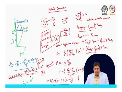
Now, in this case, In natural convection, in natural convection, what happens? There is no bulk motion of the flow, but then how the convection is happening. So, for example, you have a hot object that you place in a stagnant air, the room that is no bulk motion of the air; it is a kind of a peaceful room. And there, if you leave that object, if this object has a temperature  $T_o$ , which is greater than the ambient temperature, along with radiation, there will be the convection.
