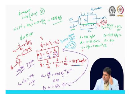
And that is why it is flown inside a pipe, the water is at 15 °C, the length is 5 m long and it is going out at 65 °C. So, 15 °C to 65 °C, we are heating water from 15 to 65 °C. The diameter of this pipe is 3 cm.
