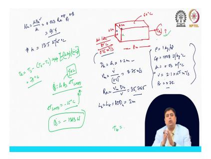
There is a heat loss happening from a duct that is say we have a rectangular or a duct of 8 m long a square duct consider in this case, which is of (0.2 m x 0.2 m) cross section. Air is going inside this duct at 1 atmosphere and 80 °C. The surface temperature of this duct is 60 °C. The temperature at which the air exit is T<sub>e</sub> so, hot air at atmospheric pressure at 80 °C enters a 8 m long duct uninsulated square duct of cross section (0.2 m x 0.2 m).
