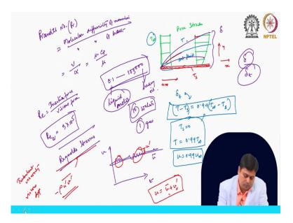
Now, at the same time when we have; so, we consider the similar situation like we have seen in case of velocity boundary layer. In that case we have seen that when a fluid approaches a flat plate there exist a boundary layer. Now, similarly when we have a hot fluid compared to its temperature is higher compared to the temperature of the solid plate, then what will happen a thermal boundary layer also will develop.
