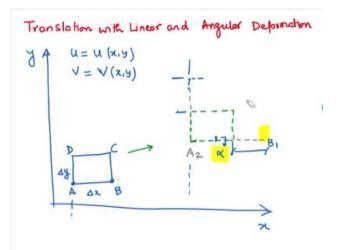
Consider a fluid element which is in a flow field, where u is a function of x and y, and v is also a function of x and y.
