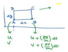
Since B has a higher x component velocity, the length of segment AB increases as time progresses. Even though B has a higher y component velocity compared to point A, the line starts to rotate or does not remain horizontal anymore. It starts to rotate with an angle with respect to the horizontal.
