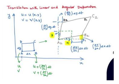
The distance between point A and point  $A_2$ ,  $l_x = u d x$ .
