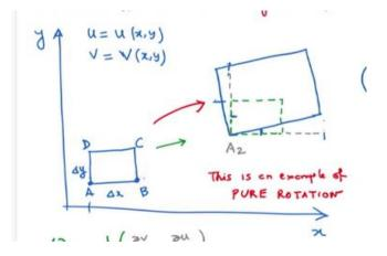
We have a fluid element which is in a flow field, where u and v both are function of x and y. For this particular condition though there is dilation since u is a function of x and v is a
