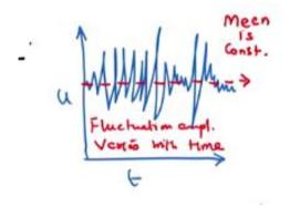
In this case, the mean velocity is nearly constant. But the fluctuation amplitude significantly varies with time.
