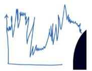
All these cases represent turbulent flow, and the four cases are different from each other by the variation of the mean and fluctuating component of velocity. So, we can distinguish or fully quantify a turbulence in terms of two velocities i.e., mean velocity and a fluctuation velocity. And this is known as the Reynolds decomposition of turbulence. Which is splitting up the flow into two parts,
