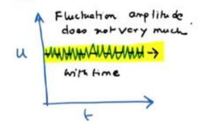
In this case, Mean velocity is nearly constant, fluctuation amplitude does not vary with time.
