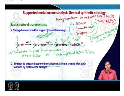
Now, what how it can be done? What can be done? Basically the fixing metallocene on support, on support means either SiO2 or Al2O3 or maybe aluminosilicates both all these combinations can be done. And theoretically three ways can be done because see in our whole system what are there we have the initiator, we have the co initiator and we have the support, support means the silica or aluminosilicates.
