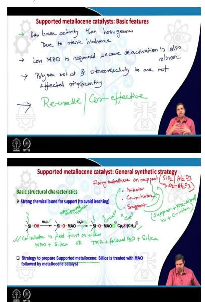
So, some of the basic features you can tell that of this supported metallocene based catalysts we can I just list down that, has lower activity then homogeneous that is obvious because you are converting to homogeneous to heterogeneous, so you have to sacrifice some the activity and due to the, this is due to the steric hindrance, if you see the, this one so here you will see there is a silica means this is a polymeric network structure.
