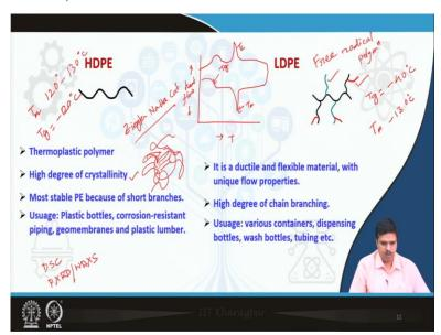
So, let us discuss in more depth. So, I already in the last class explained the classification of the polymers depending on the properties. The rubbery state, thermoplastic state, glassy state, all those things. So, here you see that high-density polyethylene, the chemical structure, the cartoon diagram is like that as I showed in the last slide.
