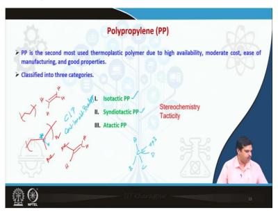
Now, the next polymers very interesting, we will discuss in quite depth about the chemical structure is the polypropylene. So, the name suggests that this is ethylene and, so this is the polypropylene. So, obviously, this is for this one monomer is ethylene and this one monomer is propylene. So, that is the difference.
