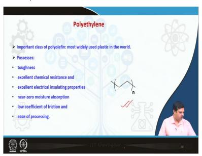
So, as I told that this is one of the heavily used polymers and the reason, the properties I already explained. This I have just pointed out for your reference. Excellent chemical resistance, excellent electrical insulating properties, ease of processing, toughness and obviously the properties are tunable, that is the mechanical strength, stiffness, toughness are tunable by changing the chemical structure and the polymerization protocol.
