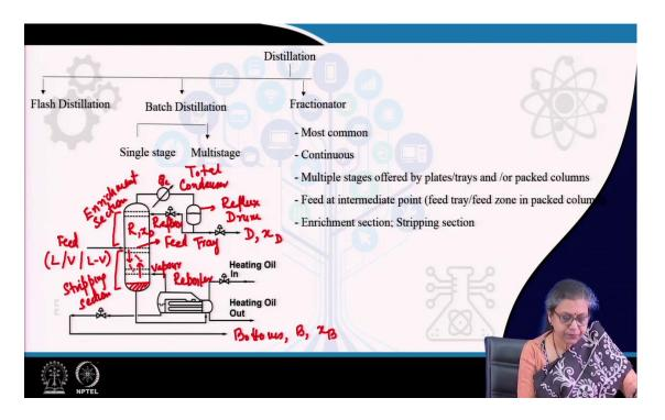
These fractionators are the most common and they are continuous processes here. There is a cascade of multiple stages that we had already discussed. Now, this cascade of multiple stages they are provided either by trays. Usually, big distillation columns whose diameters are greater than 1 meter or so, are provided with trays.
