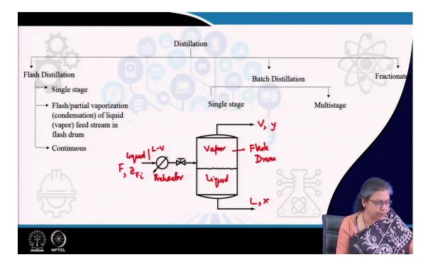
Now, distillation can be of different types. It can be a single-stage distillation, it can be a multistage distillation, it can be a batch process, it can be a continuous process.
