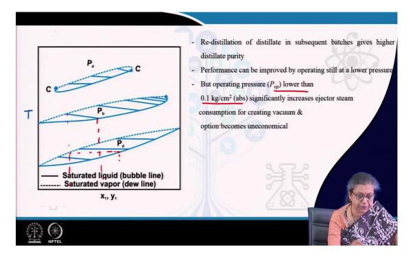
Apart from that what else we can do to improve the performance? See, it is quite evident that suppose, we go for lower and lower pressure. This particular T-x-y diagram is constructed, say at a pressure of 1 atmosphere or 1.5 atmospheres; suppose, we decreased the pressure what do we find when we decreased the pressure?
