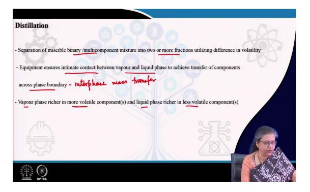
So, therefore, it is the separation of miscible or multicomponent mixtures into two or more fractions by utilizing the difference in the volatility of the components. In the distillation, two phases are first brought into intimate contact.
