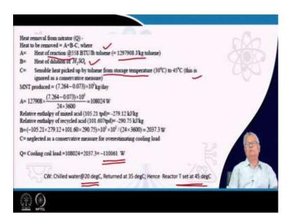
The heat removal from the nitrator is equal to the heat of reaction which is 558 BTU per pound of toulene which amounts to this value which we have talked about earlier plus the heat generated by the heat of dilution minus the sensible heat picked up by the toluene from the storage etcetera. This is in fact, ignored based on this the cooling coil heat load is estimated to be 110 kilowatt approximately.
