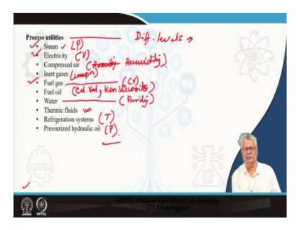
The first and foremost thing is the steam. The steam normally is either generated in a boiler or is used in various processes generated from different waste heat streams, which maybe available within the process itself. You will notice one thing in case of any process utility, there are different levels.
