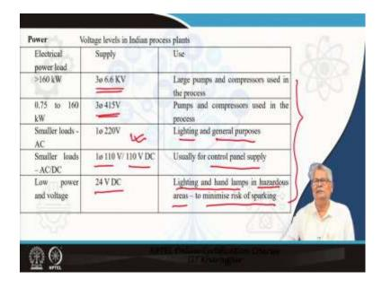
The next item that we had listed is power, electrical power; typical voltages of supply vary a lot. The most common one which we use domestically is single phase 220 volt. It is used for lighting and the general purpose, may be a fan as well. Most of the industrial pumps, they are 3 phase motor run. So, it will be 3 phase 415 volts. The pumps and compressor draw much higher power, so naturally you require a 3 phase supply.
