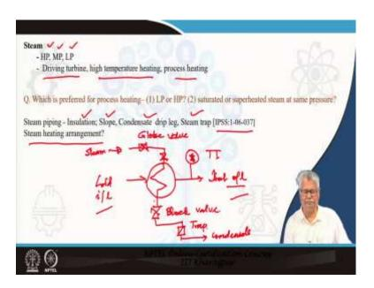
Now, we look into the details of individual components of these utilities. I mentioned that you will be having steams of different pressure ratings; typically high pressure, medium pressure and low pressure. Driving turbine normally will be done by super heated high pressure steam.
