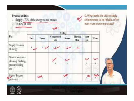
Let us look at the different utilities and their utilization. And before that, let us see and realize that in a process roughly 70 percent of the energy passes through the utility system to the process. That means it could be fuel, it could be steam, it could be power, whatever is the energy supply to the process, approximately around 70 percent of the energy passes through the process utilities.
