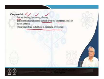
The next utility is compressed air. You usually have a supply of compressed air which you call plant air, which is used for flushing of vessels and pipelines. It is also used for leak testing; the most common way to test a leak in a pipeline, in a within the plant itself is to pressurize.
