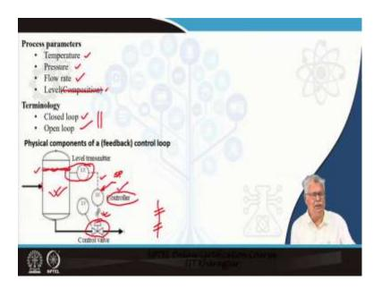
To start with, if we look at the process parameters it is very interesting that there are only four basic parameters which are involved in process control. The first is temperature, second is pressure, the third is a flow rate and fourth is a level and also composition. So, composition comes I have struck it off, but it comes at times in terms of other measurements, but it is not a very common one.
