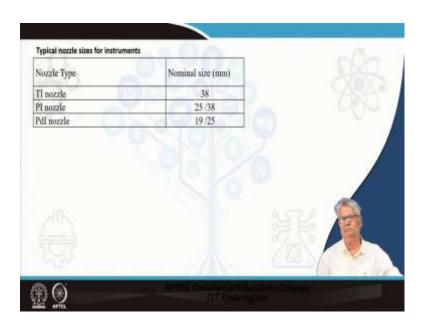
Typical instrument nozzle that also we know and we have talked about this when we talked about process vessels are 1 and a half in 38 millimeters, your pressure indication
