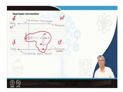
Here it is basically the same thing what you have here is a steam header instrumentation where, I have a high pressure supply this is a high pressure supply of steam this is a low pressure and you are supply you are supplying the header with your high pressure supply high pressure steam supply and a low pressure steam supply.
