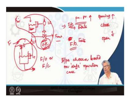
I have a vessel with a liquid which has to be maintained and there is an inflow and the inflow is while; that means, I have no control over it and it has to be served. Quite naturally I will have a level transmitter a level controller with its set point controlling this outflow from here, this is basically f in and f out this is my level controller here.
