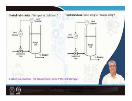
Now, you have a very interesting point here that is how to choose your control valve. We have seen that the control valve is an essential component and that is a final control element because it changes the flow and it somehow change in the flow is going to affect your pressure affect your system and here in this particular case what you find is a level control. What I do is I just look at two situations in the next slide in this slide here.
