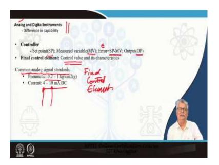
So, we move forward, these instruments particularly the controller and the sensor transmitter could be analog type. What is an analog signal? An analog signal will be taking a it can take a continuous value from its minimum to maximum. Typically, if I talk about a 4 to 20 milliamps analog signal of DC current in that case the current value could be anything between 4 to 20 in case of digital it is not so.
