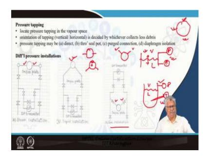
When, we talk about the pressure tappings. The pressure tappings are most of the time have to be located in the vapour space the logic is simple. If I have both vapour and liquid and I have an interface here and if I measurement my if I have my pressure measurement here, what happens is if my level varies my pressure would change.
