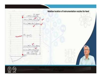
Now, what we have here is a similar thing. Here, we have a column. Normally, you will have a normal level. The level usually is measured by either a differential pressure measurement or any such thing, but normally you will be requiring two tappings; one the upper tapping at the lower tapping.
