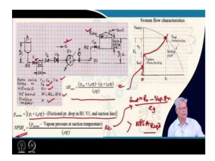
Here is an example. The example that we have here is a simple one; I have a column with some liquid level here and all my reference levels are with respect to the eye of the pump or the suction level of my pump itself. You can see z 1 is the elevation of the liquid level inside my tower, where the pressure inside at the column bottom is p 1.
