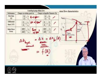
Now, we have certain relationship between the flow rate, the differential head and the brake horse power, which is basically the shaft power, which are called the pump affinity laws. The first one is, the Q is proportional to the rpm m; the second is the head or the rather the delta H is proportional to rpm square. Here what it says; the power is proportional to rpm cube, exactly the same way it is also similarly related to the diameter.
