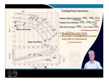
Let us look at a typical industrial pump characteristics, it is a typical centrifugal pump here. Now, what we have here is, you find that there are one, two, three, four impellers which are fitted; typically large industrial centrifugal pumps will have options of fitting a set of impeller in it. The impeller sizes will be slightly different in diameter; in this case it varies from 260 is a maximum and 222 is the minimum.
