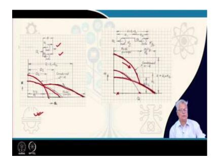
It is possible for us to have requirement of putting two pumps in series. When I have two pumps in series, naturally their heads will get added up. If I have here the characteristics of my pump 2 here and the characteristics of my pump 1 here, one thing is bound to happen. When my flow rate is less; that means I have throttled it much, both the heads get added here. But beyond a threshold of flow beyond a threshold of flow, which is this, there is no nothing to add here.
