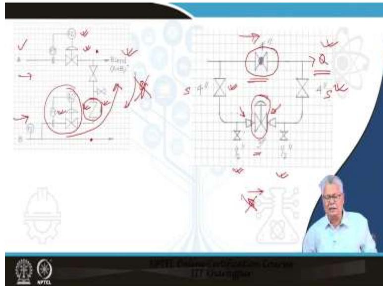
I have two more examples of piping arrangement here. Here is the typical arrangement what you have with a control valve. Let us look at the fittings. In most of the installation, what you will be finding is the size of the control valve will be at least one size, often two sizes smaller than the main piping.
