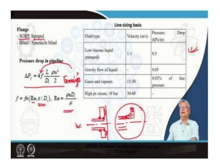
Now, we talk about the flanges the flanges the most common flanges are, if I have a pipe like this I could always have a flange mounted on this, this is a slip on type of flange it will be welded here or I could also have an arrangement of a flange which looks like this. I am not drawing the lower part it is symmetric where it will be welded here, it is basically an integral hub this is the slip on type.
