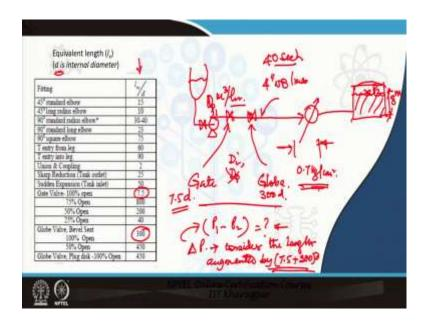
Now, comes the pressure drop in a total pipe suppose I have a distillation column from here the liquid is taken out, it has got valves here, it has a valve here both are gate valves and in order to regulate that flow I also have a globe valve here. Then what do I do I send it to a cooler cooling it, then what do I do then I send it to a tankage.
