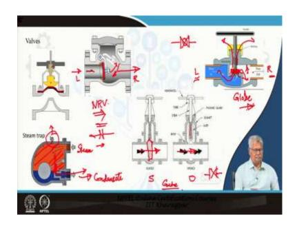
We definitely will be having valves, here we have a little I mean few types of valves. The valves can be classified as the valves which regulate a flow or the valves which either open or remain shut. For example, this is a shut valve this is the steam valve which is under open condition, what is this?
