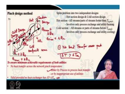
So, after this the next thing what we do is we divide the entire problem into two parts, one part is the hot section design and the other part is the cold section design right. These two designs they are divided just change it yeah. So therefore, we simply divide the
