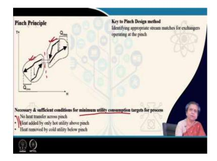
So, based on this the situation becomes slightly simpler, what we assume is that we assume that we can design the hot section as well as the cold section completely independently of one another. So therefore, we will be matching streams in the hot section and whatever we cannot match that will be compensated by the utility.
