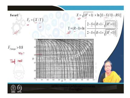
And we find out that if we go for a single shell pass which we normally prefer to do multiple two passes and singles shell passes. Then we can find out that F T can be expressed as a ratio of X and Y; where X and Y are functions of R and S the expressions are given here. So, therefore, what you need to do to find out F T?.
