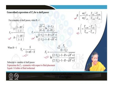
So, therefore, by convention the S is defined in terms of the cold fluid temperature range divided by T h in minus T c in and R is defined the way I have told you. So, you find that R and S both of them they are functions of the terminal temperatures all the four terminal temperatures are known to you once the terminal temperatures are known you can find out R and you can find out S.
