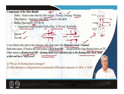
Perhaps the next question will come that how do you fix the tubes to the tube sheet? That is done in very different ways. It could be by welding for example, if this is my tube sheet and this is the end of my tube which passes through it, I could weld it here. This is not very common, but it is still there. I could use brazing also. I could also do something else.
