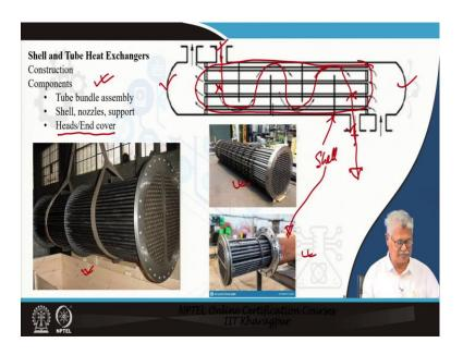
Now, what we do is let us see if we have two shells, but before that let us see look at the other components. It is the same diagram that we have here. This component is basically I have already mentioned there are tubes which are fitted to two circular discs which are called tube sheets and, the entire assembly is called a tube bundle assembly. What are the components of a tube bundle assembly? We will see just after this.
