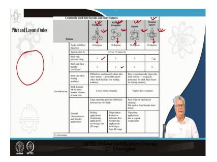
The tubes: the tubes are fitted to the tube sheet. It is a part of the tube bundle. It is possible to have within the shell or the tube sheet itself different options of layout of the tubes. It could be square as I have here, it could be rotated square, it could be triangular, it could be a rotated triangle also.
