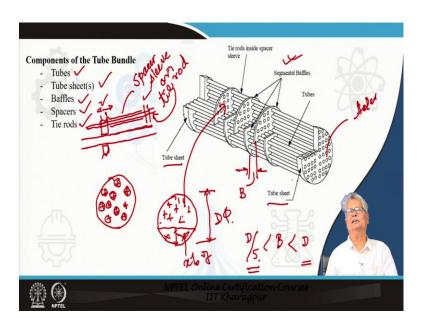
And, then we proceed now to look at the details of the tube bundle. I talked about the tubes being fitted to tube sheet which are circular sheets. Quite naturally if you have to fit a tube to a circular disc of a finite thickness we got to have holes. So, you will have holes through which you are going to insert and you are going to fix your tubes.
