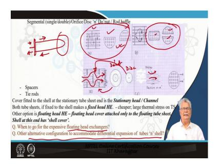
Here what we have is basically the single segmental baffles. Here every baffle set is basically consisting of multiple segments. So, it is a double segmental baffle here. So, there are three types of baffle shapes which make one pair and you can look at the flow how it takes place. Quite naturally the pressure drop in this will be slightly less.
