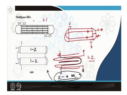
I just draw your attention to the multi pass heat exchanges. This one we know this is a 1 – 1 exchanger and I could also say that if I have a exchanger which is something like this. I am trying to draw the schematic here if I have a tube side a shell side entry from here, the shell side exit nozzle is for from this end and what I do is I have a pass partition plate which divides this particular head.
