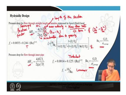
In the straight portion the pressure drop expression I did not say you have already studied this from your fluid flow, here this G is the mass velocity, what is the mass velocity? This is the mass flow rate divided by the cross sectional area. So, therefore, this is going to be this divided by the cross sectional area.
