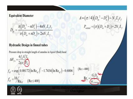
So, for the finding of the equivalent diameter it is very easy you can find out the actual area activated perimeters they are just from geometry you can find out the equivalent diameter. Remember one thing in the hydraulic design also nothing is going to change just the pressure drop across the straight length for the outer fluid is going to change everything else is going to remain the same.
