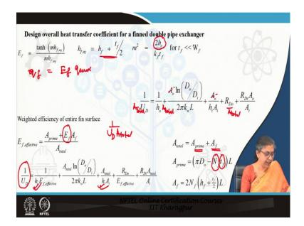
This can be this is a function of the heat transfer coefficient of the outside fluid with which it is in contact, the thermal conductivity of the fin the thickness of the fin. So, therefore, once you know m square which you can find out you know h f equivalent which I have already defined you can find out E f. Once you can find out E f you can find out q f as E f into q max right.
