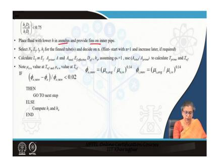
Once h i and h o are computed just check up for this. If this is fine then in if this is less than 0.75, then fluid with the lower h is placed in the annulus and fins have to be provided. Remember one thing usually fins are provided on the outer surface it is very rare to have fins on the inner surface.
