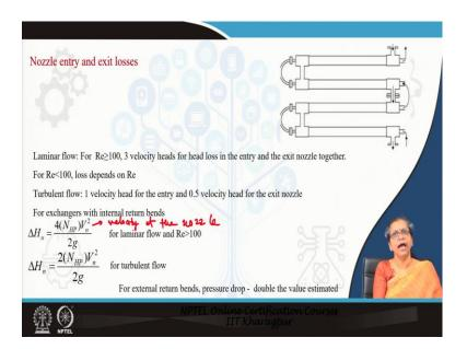
Same way the same type of expression it is applicable for the case of the head loss at the nozzles as well, in this case also it is primarily for the outer tube and for the inner tube we take it to be negligible and this gives you the velocity at the nozzle or this gives you the nozzle velocity right.
