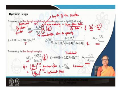
So, therefore, we often here we give some particular correction factor here, we often multiply this with some particular correction factor here where this particular phi this is equal to mu by mu w to the power 0.14 for laminar flow and this is equals to mu by mu w to the power 0.25 for turbulent flow. So, very frequently when we find that the
