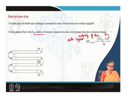
Now, for the bend portion. As I have already mentioned for the inner pipe the bend pressure loss is usually negligible and for the annular fluid suppose there are N HP number of hairpins then naturally the number of bends will be NH 2 N HP minus 1 right. So, therefore, from here we can find out the head loss at the bend where this particular V o this is nothing but the velocity of the outer fluid.
