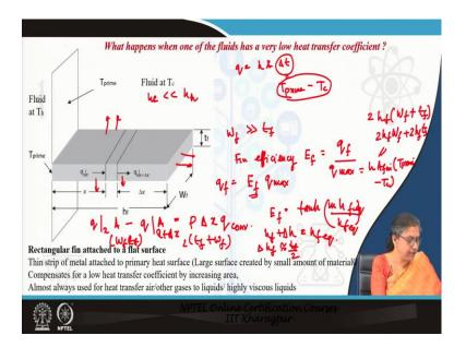
How do we increase the area just as I have shown you that in that case one thing we can do, we can increase the heat transfer area. Now, a very simple way of increasing the heat transfer area if you see in this particular case, say this is the separating wall we have a fluid here I assume that the fluid which I have here that is the that fluid is at a higher temperature, say as you and this fluid is at a lower temperature and this is the heat transfer area.
