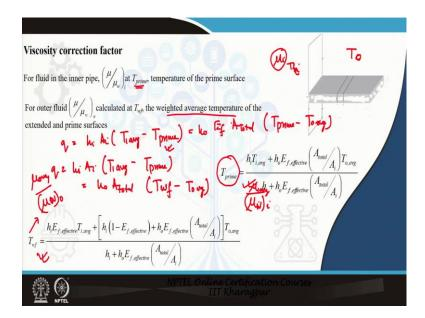
Now, for the viscosity correction factor as I have already told you that this particular viscosity correction factor it has to be defined with respect to the wall temperature. What is the wall temperature if you see? For the inner fluid say if it was at T h, the wall temperature is the temperature at T prime what is the temperature the wall temperature for the outer fluid? This has to be some sort of a weighted average temperature of the extended surface and the prime surface right.
