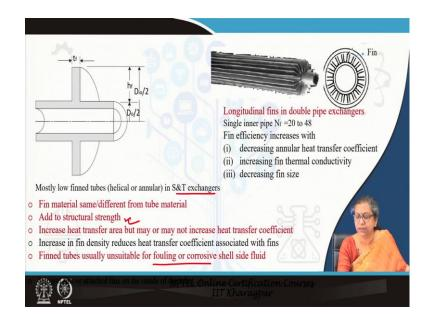
Well. So, therefore, now you have understood that for these particular cases where we have one particular fluid which is at a much lower much has a much lower heat transfer coefficient what we do? We try to increase the surface by means of fins, but remember one thing fins they increase the area, but they may or may not increase the heat transfer coefficient and the increase in heat transfer rate that will depend upon the fin effectiveness.
