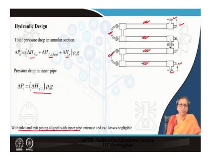
Now, you tell me to find out the pressure drop what are the things that you require? Very clearly if you see this particular exchanger arrangement that I have the drawn here, the most conventional arrangement, the series arrangement of two hairpins where there is counter current flow of the outer fluid as well as the inner fluid.
