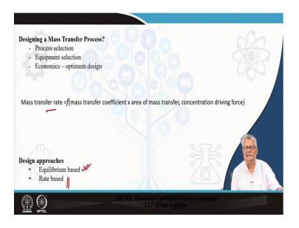
Whenever we are talking about designing any mass transfer process, these are the steps. First, most of the mass transfer processes are basically separation processes. So, we got to select the process; that means, whether it is distillation or absorption, adsorption, extraction, leaching or whatever type of process that we have, that we require in order to make the separation that we have to decide.
