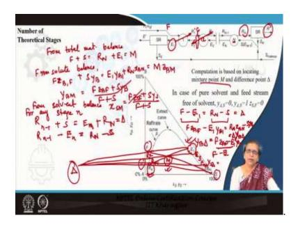
So, now see just like we are done for absorption and distillation in this particular case also what we do we perform this particular stage calculation based on the overall material balance and the component material balance. So, from the I have drawn the diagram here this is F and it goes on this the from the last stage N th stage R N comes in and from here S enters which is nothing, but the extract entering from the N plus 1 th stage and what comes out is E 1.
