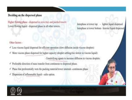
But in this particular case it is very interesting to note that in the case of sieve trays and packed towers the phase with the higher flow rate is dispersed and for all other the towers the phase with the lower flow rate is dispersed. Next thing is relative viscosity, this is something very interesting.
