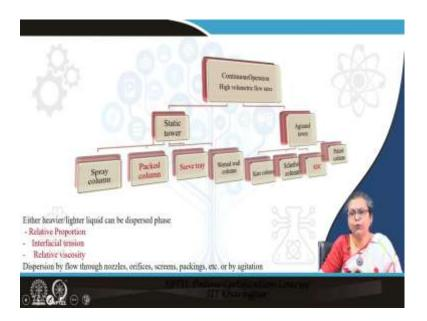
Now, as I have mentioned to you in this particular case what do we do? For continuous operation columns be it static be it agitated there is a heavier phase there is a there is a lighter phase. The heavier phase comes, the lighter phase rises up, the heavier phase comes down and one of them is going to be dispersed as droplets into the other. This dispersion as we have found we can use nozzles, orifices, screens etcetera and we can also enhance this particular dispersion by means of agitators.
