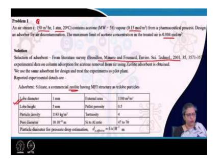
Well. So, with all these things now I think we are in a position to just look into a typical problem of adsorber bed design we start with the gas phase adsorption. What do we have? What is our feed? Our feed is an air stream, the flow rate of the air stream is provided, the feed condition is provided.
