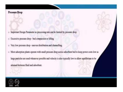
Now, this pressure drop as I had mentioned in the last class, it is something a very important parameter because the processing rate it can be limited by pressure drop and if you recall, if you have a very high pressure drop what happens? It can result in the lifting of the bed or it can result in the bed compaction depending upon the direction of the fluid flow.
