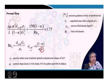
So, therefore, in this particular case also we use Ergun equation. I have listed down the nomenclatures of each and every terms that have been used here along with the relevant dimensions.
