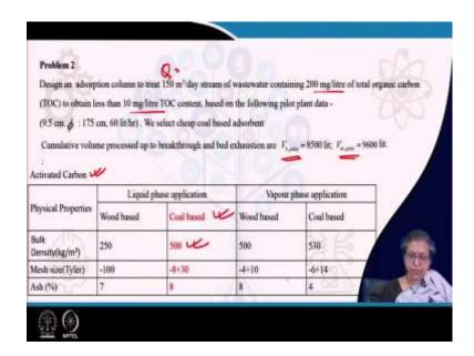
In the same way I had I will just touch upon another adsorption problem for waste water treatment. Again in this particular case the total Q is provided, the initial concentration is provided, the permissible concentration is provided. Since this is wastewater treatment if you recall that activated carbon was a potential source. So, we select activated carbon and from the table that I had shown you, I go for a coal based activated carbon from where I select this particular bulk density.
