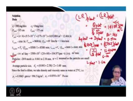
So, therefore, here I have listed down all the different data which are available for the pilot plant and also the flow rate etcetera the particle dimensions everything has been put down here. From there first what I will do? I find out the LR plant. LR plant what is the LR plant? This is equals to the LR pilot what is the LR pilot? It is Q pilot by the cross sectional area of the pilot plant.
