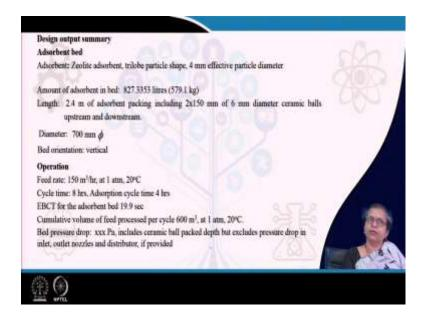
After it was completed then more or less the design summary has been put up in this particular form where the total amount of adsorbent the length and diameter etcetera etcetera all those things are there, the only thing which is remaining is the design of nozzles etcetera which we will be taking up when we go for the discussion on the pressure vessels. So, this was a typical problem for gas adsorption.
