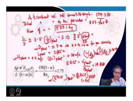
So, from this if you can find out the adsorbent volume which is necessary till breakthrough. We can find this out and once we can find this out we can also find out total adsorbent volume to be provided. What will that be? That is going to be suppose the adsorbent volume till breakthrough it is near about equals to say 554.3 liters just check up these particular quantitative measures.
