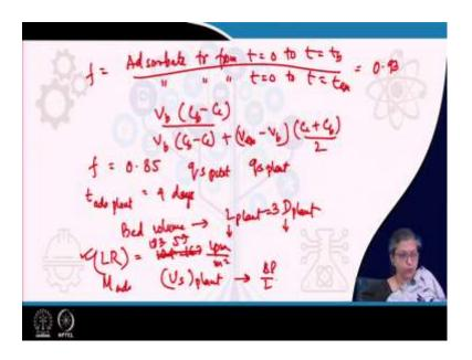
If we assume that the curve was more or less symmetric then in that case we can find out the f from the adsorbate transfer from t equals to 0 to t equals to t b divided by adsorbate transfer from t equals to 0 to t equals to t exhaustion. From there if you find it out you will find that it is nearly equal to 0.93. This adsorbate transfer this is nothing, but V b into C b minus C i divided by V b into C b minus C i plus V exhaust minus V b.
