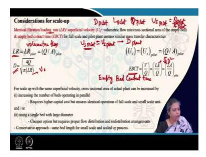
What are the data that we have on the pilot plant? We know the column the pilot column dimensions, we know the D pilot, we know the L pilot, we know the Q pilot, the flow rate of the feed through the pilot plant. So, we know all these things. So, definitely when we know these things, we can find out the U s pilot. It is nothing but the Q pilot divided by the cross sectional area of the pilot.
