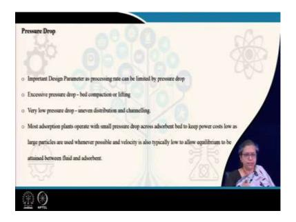
So, once we have done the design more or less then we go for the pressure drop part. The pressure drop is something very important which you need to remember. Why? Because if ressure drop is excessive then it leads to bed compaction or lifting, if the pressure drop is very less then there will be uneven distribution and channeling.
