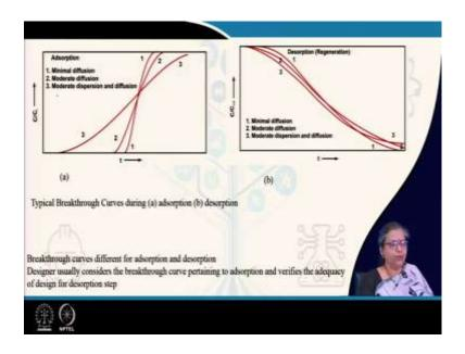
There is just one thing which I would like to mention, see when you are having the breakthrough data you will find that different curves are generated for adsorption and for desorption. So, for the design what would you have to do? For the design we would generally consider the breakthrough curve which has been generated for adsorption pertaining to our specific situation and then we will verify the same for the desorption step.
