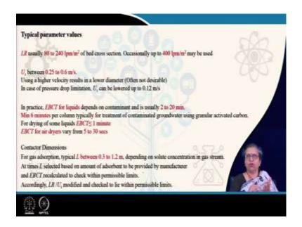
And we would also like to check up at the end - the empty bed contact time and also the loading rate, the superficial velocities; these particular values normally for industrial adsorbers have been observed to lie within certain ranges.
