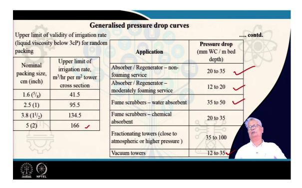
To generalize pressure drop curves which we have presented in the two slides before this, we also have something. We have an upper limit of irrigation rate was shown to you earlier is dependent on the packing size and why it is so, that is explained earlier as well.
