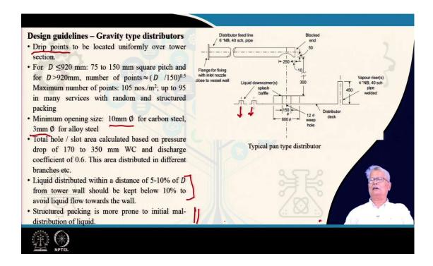
What we have been discussing in the last class is regarding the gravity type of distributor, where we have seen what are the different components and what these details are. The first thing here is the drip points. That means, we have to have the weeping arrangement and also the drip points means these are the drip points and they are to be located as uniform as possible.
