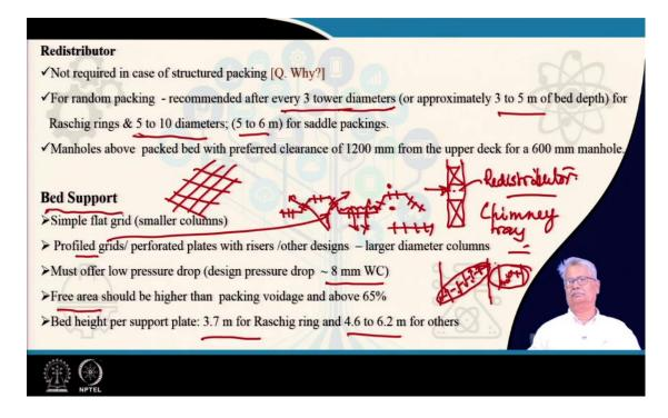
We have talked about the distribution. In some cases, you require a redistributor. Suppose I am talking about a column in which I have two sections and I have feed entry in between or even if I do not have I require a very large amount of packing
