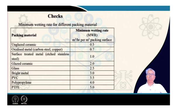
There are a few checks that you got to make. The minimum wetting rate for different packing materials needs to be checked that you remain within. I mean you remain above the minimum wetting rate and you are utilizing the entire surface of the bed which is available for your mass transfer.
