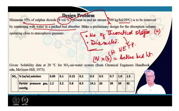
Before we go into the design of the packed towers, let us look at typical design problems as are faced. Here we have a design problem that simply says that a minimum of 95 % of sulphur dioxide is present in the air stream. I could have put it like this.
