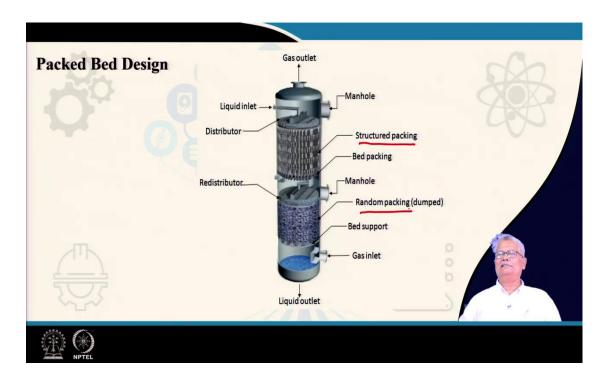
This is the diagram which we have already seen earlier where you have a typical demonstration pack tower and what are its components. Quite naturally the gas is exiting from the top and the liquid is distributed from the top itself through the liquid inlet and it comes out from the bottom and here it as it shows you have a redistributor.
