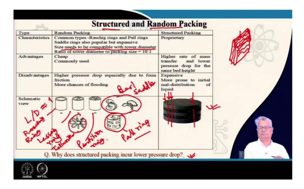
We have been introduced to the structure and the random packing. Random packings have different characteristics, advantage, disadvantage and there are different types. Here L/D of this cylinder is nearly 1. This is a Raschig ring. There is a partition in between, this is a Lessing ring. You have a cross partition here. So, this is called a partition ring.
