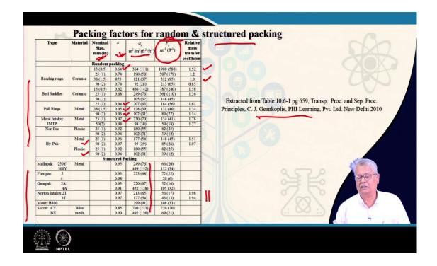
This is a very important characteristic of the packing that you have. The different types of packing are set here. The different types of random packings are here. Raschig ring, berl saddle, pall ring, metal interlocks IMTP, Nor-Pac, Hy-Pak and all these are proprietary ones and these are all random packings.
