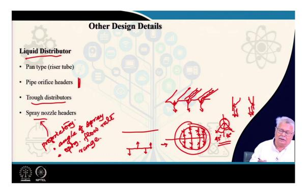
Now, you need to know about the other design details. The liquid distributor in the case of a packed bed is very important. We talked about the different types of distributors. The spray nozzle header is very very simple basically what you have is if you have a tower in which you have to spray you definitely will be having this type of branch coming from a liquid entry distributor and you will have your sprays located here.
