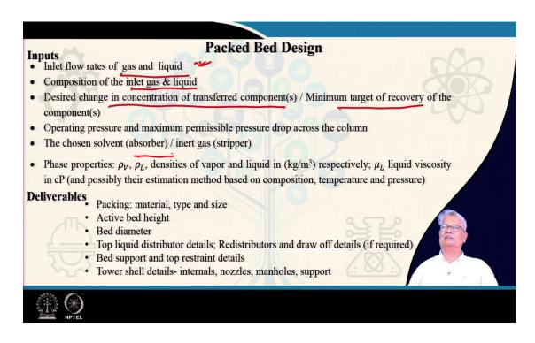
You have been supplied with a design problem. What are the inputs? These are the inlet flow rates of gas and liquid. Yes, you already have found out how to find out the minimum amount of liquid required. Based on the minimum liquid, you have assumed about 1.5 terms of that liquid rate and possibly by definitely by this time when you have come to the design of the bed itself you know what are the inlet flow rates.
