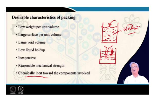
Now, let us look at the desirable characteristics of the packings. The packing has to be supported. So, the lighter the packing the better it is. So, lower weight per unit volume, when I say unit volume it means, the packing packed bed volume.
