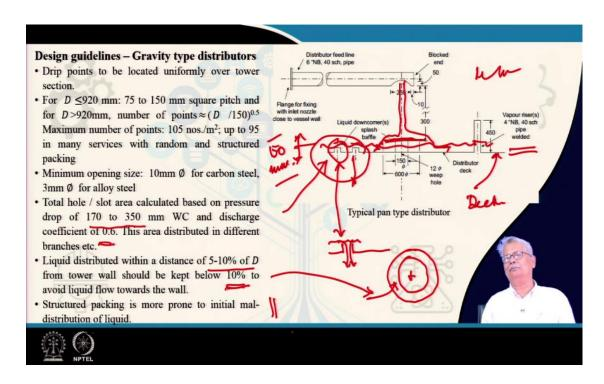
This is something which we have discussed earlier and this is the simplest type of distributor which you use and what you have here is a pan deck. Basically, this is your deck with liquid downcomer; that means, on the deck, you will have a liquid and the liquid will flow through these.
