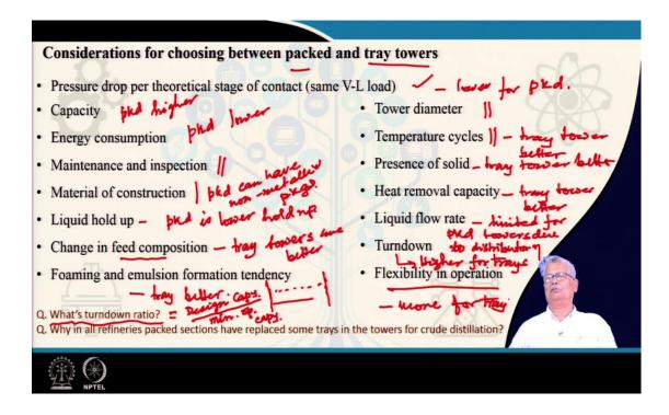
To start with, we need to know that what are the basic considerations for choosing between the packed and the tray towers. So, we have two options of vapour-liquid contracting that is what we have been focusing on and we need to find out the advantages and the limitations of each type.
