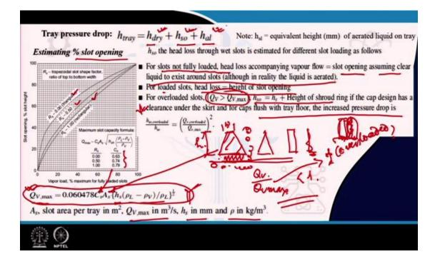
Next what we do is basically, the same thing we have to estimate now the percentage of the slot opening; because the pressure drop which is encountered at the slot outlet as the vapour comes out will depend on how much opening it is present there.
