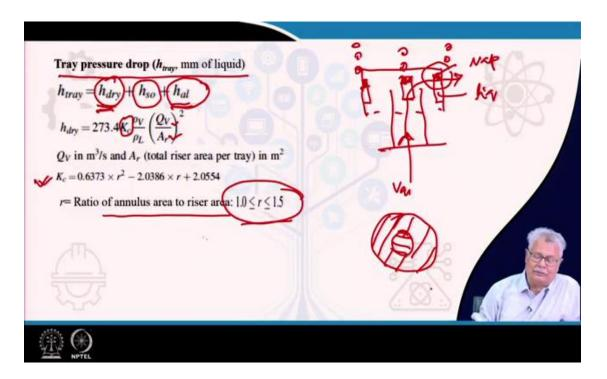
Remember this is a technique I mean this technique is valid only for bubble cap trays. This particular correlation. The third part that we are going to deal with is the tray pressure drop, which is h tray, which is going to be expressed finally in the mm of the liquid which is there on the tray itself.
