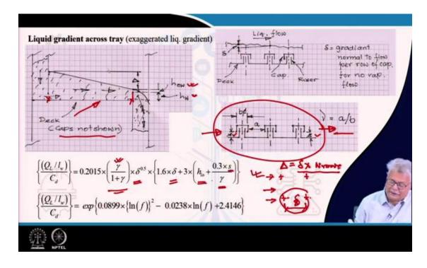
If my tray has to operate smoothly and without any channelling of that vapour going through that inner layer of liquid, we must have as low a difference in the level of liquid over the tray.
