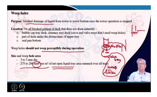
The purpose of a weep hole is gradual drainage; that means when my operation stops from the tray I want everything to come, all the liquid to get collected in the column bottom. And why it happens, we just explain that. Now, this draining will be necessary where? It will be needed on all blocked portions of the deck. That means where it does not drain naturally or freely. What are these places and locations?
