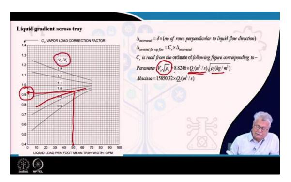
I have redrawn the same thing here. The  $V_0\sqrt{\rho_v}$  is what? The  $V_0\sqrt{\rho_v}$  is basically the volumetric flow rate multiplied by rho v and I have already converted the constant so that
