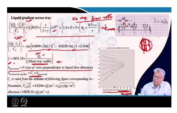
Now, you have here is basically h, what is  $h_{lo}$  at a height of liquid over the weir? So, all these are here. There is another way to express or find out the same term in using another expression, which uses a parameter small f. The small f is related to the frictional drop.  $Q_L$  is the flow rate of liquid across the tray and you have a mean tray width.
