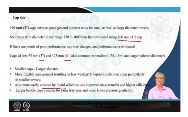
The most common industrial capsize is 4 inches, 100 mm. It is usually the most popular type and it is used in small towers as well as large towers. Normally, if you are going to expect that the diameter of your tower is going to be slightly less than a meter to around 3 m. You can try by checking with the 4-inch caps first.
