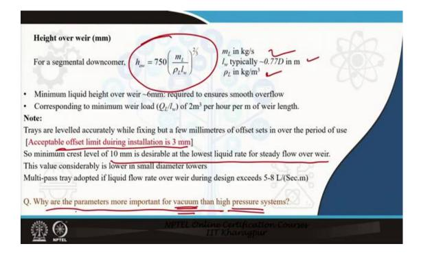
The height over the weir in this case also is given by the Francis formula with proper units that you must note from this. Corresponding to the minimum weir load, we usually try to keep at least 2-meter cube per hour per meter of weir length.
