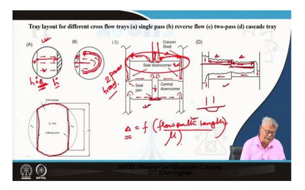
Now, we can have various types of layouts on my tray. This is the simplest. We have a single downcomer and a single pass. The flow path length is from here to here, it goes like this. We have a gradient of liquid level at this point and this point. It flows by gravity. So, naturally, the h here will be  $h + \Delta$  and if my h is here. This  $\Delta$  is a driving force for the liquid from this point to this point.
