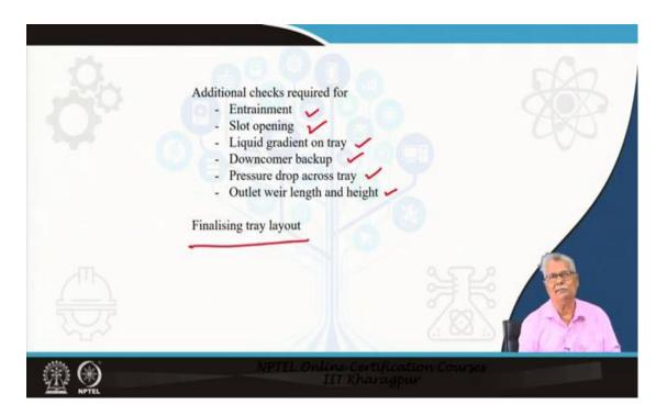
Slot opening, liquid gradient on tray, downcomer backup, pressure drop across tray and outlet length outlet weir length and height. Definitely, we have to finalize the tray layout; that means, where to place the vapour disperses.
