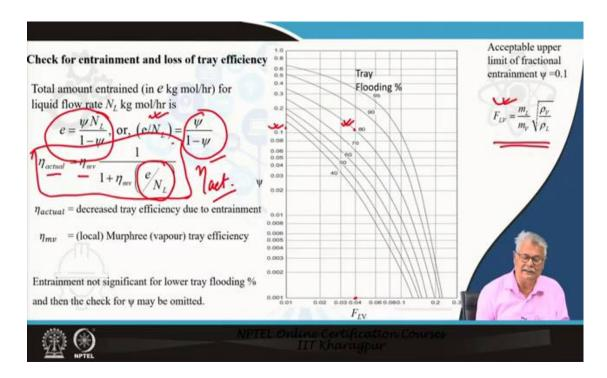
To start with we talk about entrainment. This entrainment check is also very similar to what we have seen. It is practically the same as what you find in the case of your sieve trays. It is the same plot. The same  $F_{LV}$  factor is used which is the ratio of mass velocity of liquid to mass velocity of vapour. Then you have the  $\frac{\rho_V}{\rho_L}$ . So we know the value of  $F_{LV}$ .
