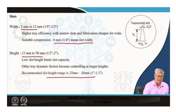
The slots width typically be either I mean will be normally 3 to 12 mm wide. The suitable compromise is a 6 mm mean slot width. The height of the slot can vary depending on the size of the cap from 12 to 50 mm. The recommended slot height ranges 25 to 38 mm. 38 mm mean 1 and a half-inch.
