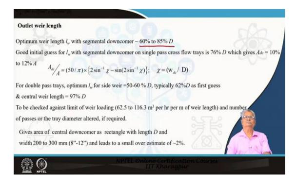
The bubble cap material typically is 410 SS 410. Now we have to have an idea about the optimum weir length with the segmental downcomer. The segmental down comer typically the length is around 60 to 85 D.
