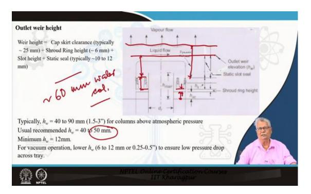
Now, there is a very important point here. I have to have my vapour dispersers submerged in the liquid. So, we provide an outlet weir for this and the weir height is based on, you can see and you can add from here directly. It is a caps skirt clearance; the caps skirt clearance is this distance. The shroud ring height; the shroud ring height is this distance. The slot height; the slot height is from here to here.
