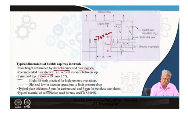
Now, what we have is basically about the typical dimensions of the cap tray internal. We have to specify the riser height. The riser height is determined by the skirt clearance and the riser slot seal. We know what the slot seals are. And the recommended riser slot seal that the vertical distance between the top of the riser and the top of the slots. This is typically 38 mm which is about one and a half inches.
