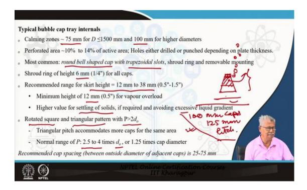
To have the layout, we need to know about the dimensions which are typically used. The first thing is a calming zone. Typically, if the diameter of the tower is below 1.5 m. You
