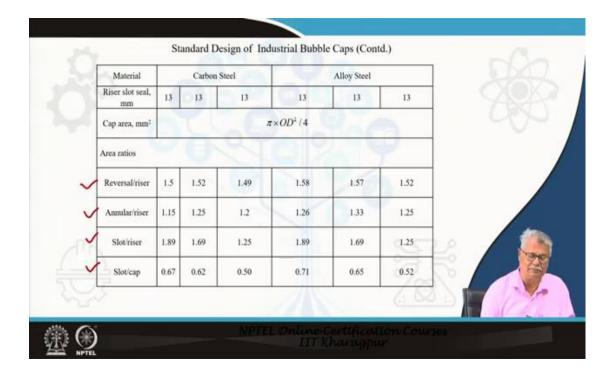
These are the other details which is given here and the different area ratios are there. Because this area ratio are required when you go for your design and you need to calculate your other parameters regarding the flow hydrodynamics around your bubble cap.
