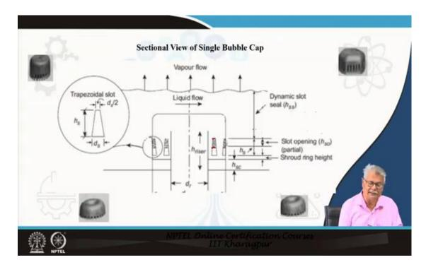
Now, what we do is, we look at the view of a double bubble cap and it is the same thing which we have here and all during our design. We are supposed to find out the slot opening. That means when it operates by how much will the liquid level here in the slot get depressed. We definitely will have to check this and we move on with this.
