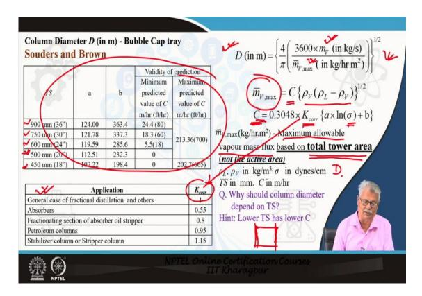
Now, we need to find out the diameter. There are two techniques for finding the diameter of bubble cap trays. The first is proposed by Souders and Brown. This is a very standard and classical procedure. The procedure depends on or rather relies on an empirical relationship of estimating the  $\overline{m}_{V,max}$ . The  $\overline{m}_{V,max}$  is the maximum allowable vapour mass flux. I have put in bold that it is based on the total tower area, it is not the active area.
