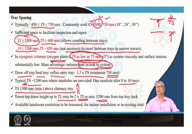
Now, there is something. If you are making a column, tray spacing directly influences the total height of the column that means the column cost. Typical tray spacing lies between 450 and 750 mm. Most common is in fact, 600 mm. Typical standard values are 450, 600, 750 mm. You can have lower tray spacing also particularly in smaller columns.
