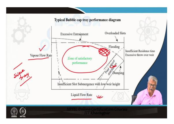
We will go further and have a look at the functioning of the bubble cap over the zone of liquid flow rate and the vapour flow rate. This is very similar to what you have seen in the case of the other disperser which is basically your sieve tray. What you find that in this case also you would like to maxima. You have a zone of satisfactory performance.
