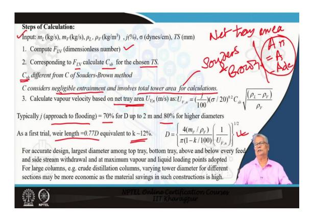
The steps of calculations, in this case, are the compilation of the inputs. Computing the  $F_{LV}$  value, corresponding to  $F_{LV}$  estimating the  $C_{sb}$  for a chosen TS. We will note that here that the  $C_{sb}$  values are different from the C of the Souder-Brown equation. C considers negligible entrainment and involves a total tower area for calculation. This is a major difference what you have.
