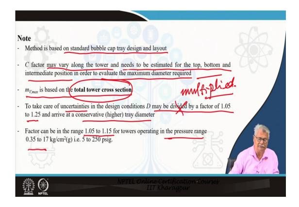
The Souders-Brown method is based on the design of standard bubble cap tray design and layout. The C factor may vary along with the tower and needs to be estimated for the top, bottom and intermediate positions. So that the maximum diameter required in a particular section is determined and normally, that is the tower diameter which is kept for the other trays which may or may not require blanking of certain of the vapour dispersers.
