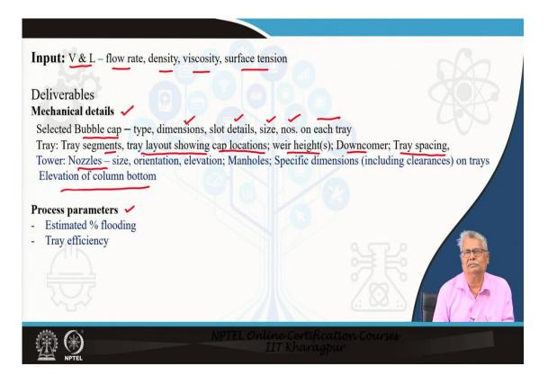
First, we see one thing that in case we have to design a tray, the basic inputs that are required are the vapour and liquid related items like the flow rate, the density, the viscosity and the surface tension. These are the four things that you require. If you are talking about the deliverables, there will be two sets of deliverables, the one set will be the process parameters.
