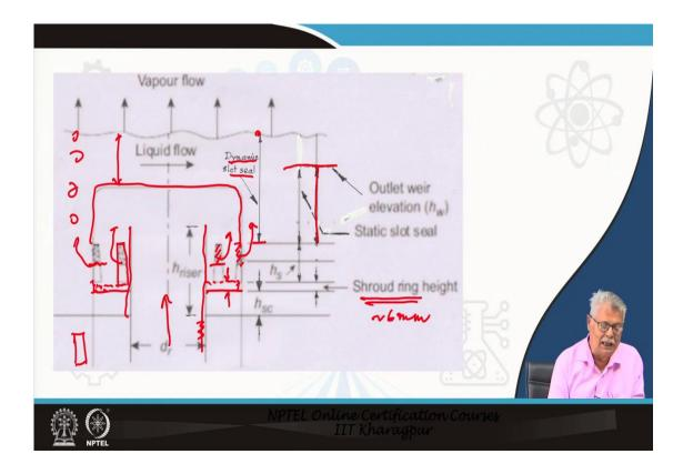
Let us have a look at the bubble cap first. This is the cap. This cap is mounted on a riser. This part you can forget. The vapour goes up this way, comes out through the slots and bubbles up. The mechanism of working we have seen but let us see to function properly. Certain essential things have to be obeyed.
