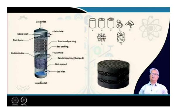
This is also something which we have seen in the last class. This is about structured packing which comes in blocks. These blocks are sewn together and put inside. The random packings are dumped. Various random packing shapes are given here with distinctive names. I am sure that you have come across the individual names while you have started your packed towers in your mass transfer course.
