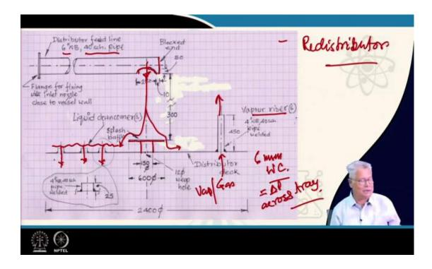
Here is the last part, which means, we are talking about liquid redistribution. Now I have answered one of your old questions that is if I have to redistribute, I have to collect the liquid. The collection of the liquid could be done using a chimney tray. The redistribution is what I am going to talk about right now.
