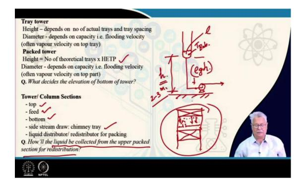
We took a few main features of the tray tower. The height which depends on the number of actual trays that are to be provided and the tray spacing which in most cases will not be uniform all through. There will be two sets at least. Some trays for example like the feed zone and the top one will have different tray spacing.
