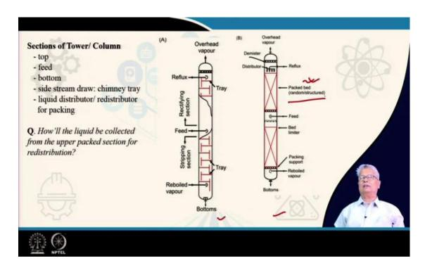
The sections of a tower are the top, feed. We still have the question. We have here the same old diagram which compares the different sections. We also have one additional thing that reminds us that packing for us could be a packed bed which is random or structured. Possibly, we will have structured packing these days because structured packings though more expensive than the random ones, they are they offer lower pressure drop, and higher specific area of contact.
