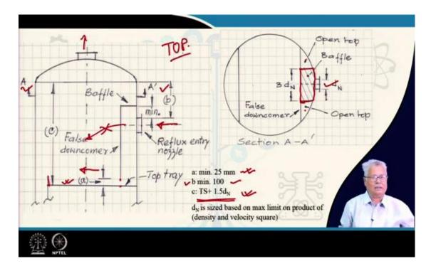
We look at the different sections with dimensions. This is the top section of the tower. This is my top tray. Here in this top section, you will have a vapour outlet. You will have a reflux entry here. The vapour is supposed to be fully vapoured. You may have or you may not have a demister at the top. The reflux entry is supposed to be for a liquid flow rate. So, if I have to provide the dimensions of this, let us understand all are the physical arrangements made here.
