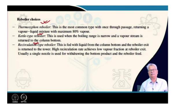
Now, you can have different reboiler choices. You have read about this in your mass transfer. You can have a Thermosyphon reboiler, you have Kettle reboiler, you have recirculation type of reboiler. The basic difference between is their construction. In Thermosyphon what happens, you have a vapour plus liquid recycled, the most of it is vapour.
