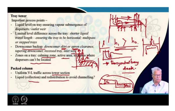
In the case of a tray tower, there are certain important process points. We have distinguished between the cross-flow trays and the only type of counter-flow tray that we have come across is the sieve tray without a downcomer. But, in the case of cross-flow trays, the liquid will be coming from the upper tray will be flowing out like this, flowing over a weir, and going this way, this is the downcomer of the tray.
