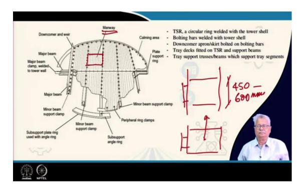
This is again the tray tower. Here, in my last class, I have forgotten to mention about one very important piece. We said that these are segmental decks. The decks are made in the segment, inserted through the manhole and assembled inside. You have typically in towers the tray spacing is anything between 450 to 600 mm. Quite naturally this has to be fixed. If this has to be fixed, then what happens is someone has to go in here.
