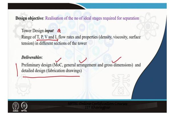
Now, I show you here that the purpose of the practical tower is the realization of the number of ideal stages which are estimated to be required for the separation itself. Now, in order to do it, you shall be requiring the temperature, pressure, volume, and liquid flow rates, and also gas flow rate, and properties in the different sections of the tower.
