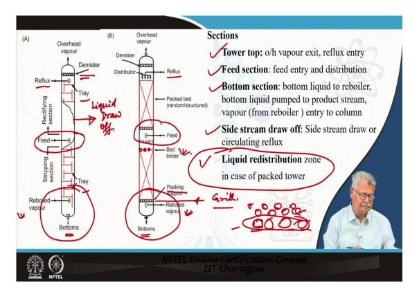
Let us look at the various sections of these two towers. The left one, obviously, is a tray tower – you have trays here. On the right side, you have a packed tower. If you are talking about the packed tower, the packing requires support because it has its weight has to be supported by something strong. So, often you will have a pack.
