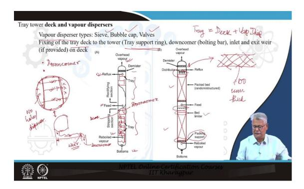
We look at the tray tower and packed tower general arrangement. We talked about dispersing one phase into the other. Conventionally in tray towers, the vapour is dispersed and depending on the type of arrangement we have for the dispersal. It will be a sieve tower which means you just have a hole. It could be a bubble cap where you have an inverted cup-like structure over a nozzle or a riser or it could be valves that have got a movable part also.
