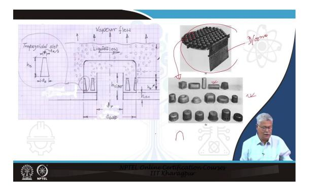
Here what you have is the diagram of a bubble cap tray. The different types of bubble cap trays that are used in industry are given here. You can understand this is the complete tray. This part of it is the down-comer. These are the vapour dispersers in the form of a bubble cap. Though we have said a bubble cap should look like just a cap there are different shapes. It doesn't have to have a circular shape. It could be a rectangular one also or something similar to that.
