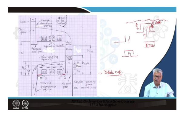
This is again basically the arrangement with a typical type of vapour disperser which we will be contacting and we will be learning the design of this. This disperser is the bubble cap disperser. What it is? It is nothing, but a riser that is fitted to the tray covered with an inverted cup.
