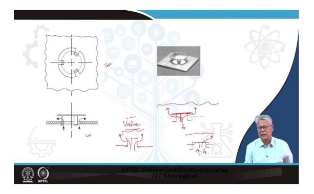
So, beyond this what we see is the other type of disperser. The other type of disperser is the valve type. The valve type means basically what you have in this case is a flat disk. The flat disk if it sits on this hole, it will close the hole. So, and you have the gas which is pushing it up and it emerges in liquid. A gas goes like this, forms bubbles and it comes out.
