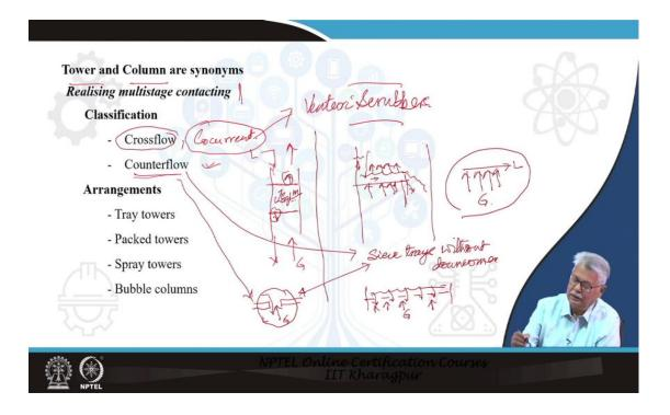
Now, I repeat once more that we are going to use the terms tower and column to be equivalent. What are they used for? They are used for realising multistage contacting. That indicates that in the same piece of equipment, you are expected to provide more than one ideal stage of contacting. Now, so far we already have seen in the case of heat transfer class or mass transfer class that counterflow gives you, in case of contacting of two species, a higher driving force.
