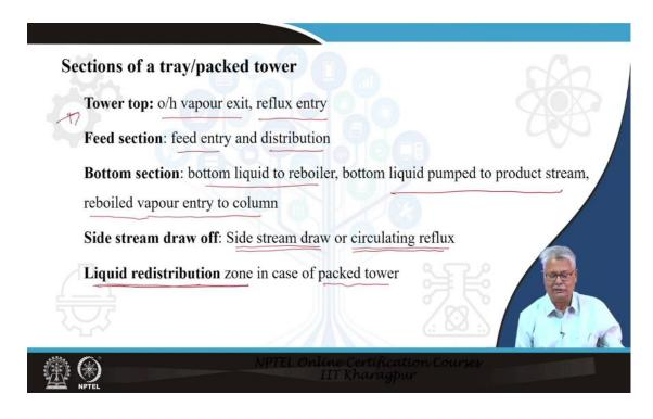
When we talk about the different sections of a tray or packed tower, we have to have the details of different sections. We focus on different sections. We have divided the sections which are common for all types of dispersers and in the case of the packed tower also.
