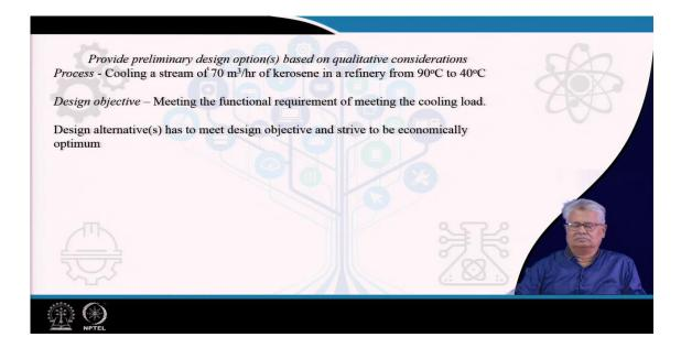
We have a very simple case. We have here a preliminary design problem with us where the processes of cooling a stream of 70 m<sup>3</sup>/h of kerosene, which is available in a refinery from its initial temperature of 90°C to a final temperature of 40 °C. Typically, most of the processes before their storage, if it is a light material is standard to cool it up to 40 °C before sending it to the storage.
